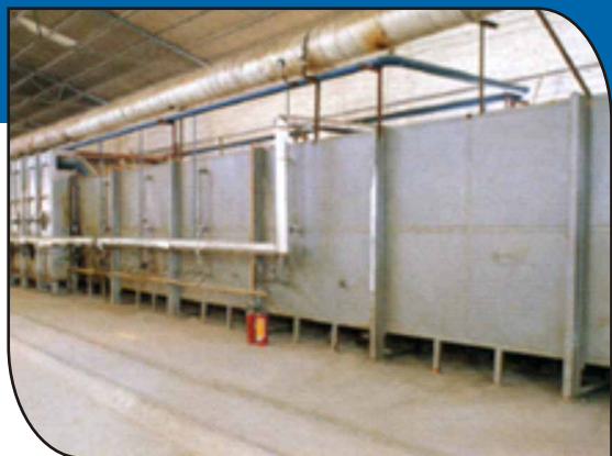
Kiln suitable for firing at 1650° C
