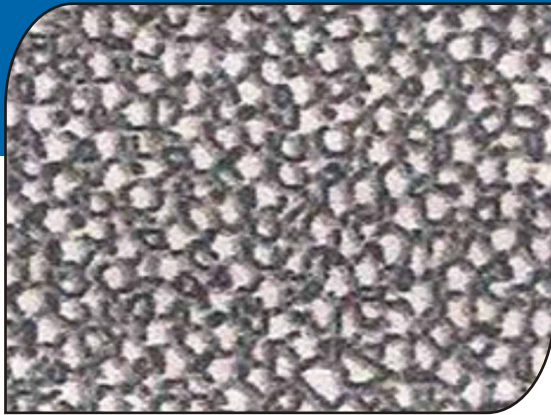
With low SiO 2 and MgO, White colour (Chemical Grade Alumina) Sintering Temp. 1520 Deg.
