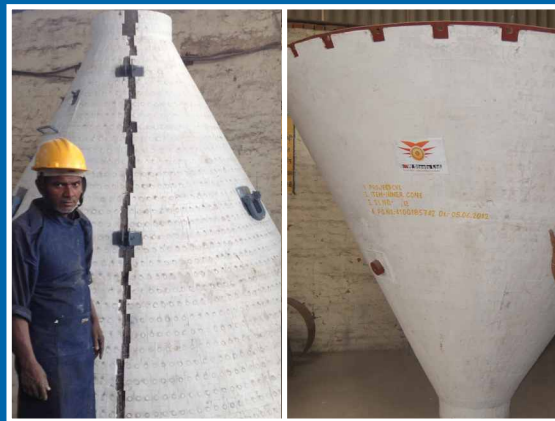
Both Side Ceramic Lined Inner Cone in 3/4 Pcs
