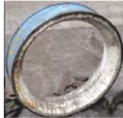
Eroded Fixed Orifice
