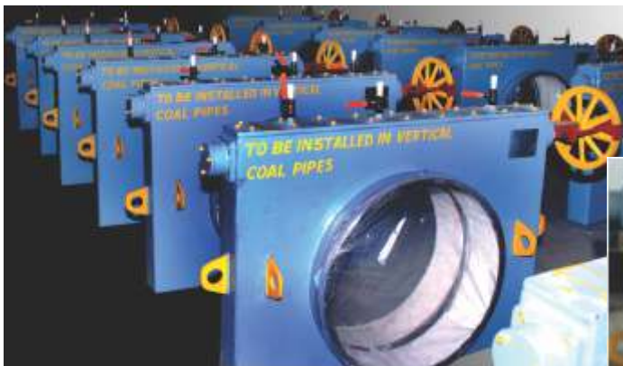
Alumina Ceramic Lined Variable Orifice 100% open
