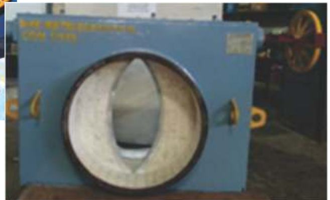
Alumina Ceramic Lined Variable Orifice 40% open
