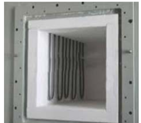
Lab Muffle Furnace (1700Deg C)
