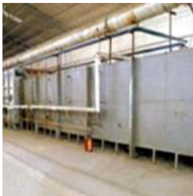
Tunnel Furnace (1550°C)
